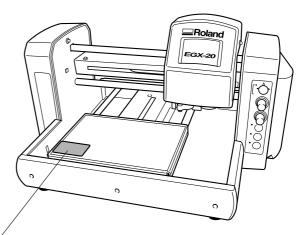
Place the plate on the adhesive sheet, then press down on it from above to anchor it securely.
